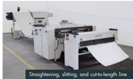
Straightening, slitting, and cut-to-length line
