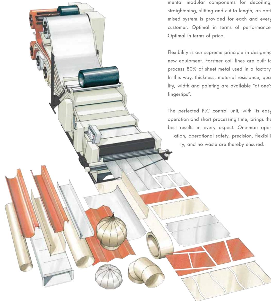
The requirements of our coil lines are just as varied as the daily working practice of our customers. For this reason, Forstner lines are not available "off the shelf". On the basis of fundamental modular components for decoiling, straightening, slitting and cut to length, an optimised system is provided for each and every customer. Optimal in terms of performance. Optimal in terms of price.
