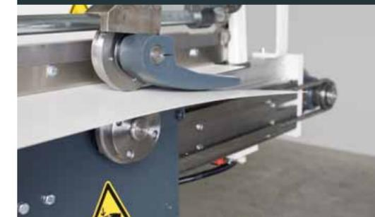
Cutting to length with manual/electric slitter or guillotine and additional functions can be added for example recoiling
