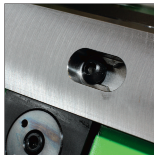
Quick change of tooling (bayonet style) and adjustable crowning.
