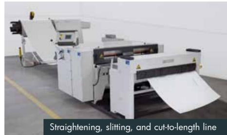
Straightening, slitting, and cut-to-length line
