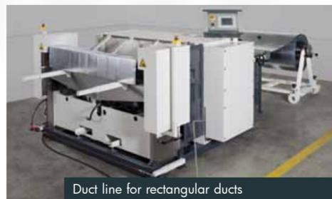
Duct line for rectangular ducts
