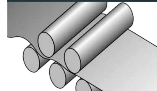
Straightening of the coil set with three or more straightening shafts
