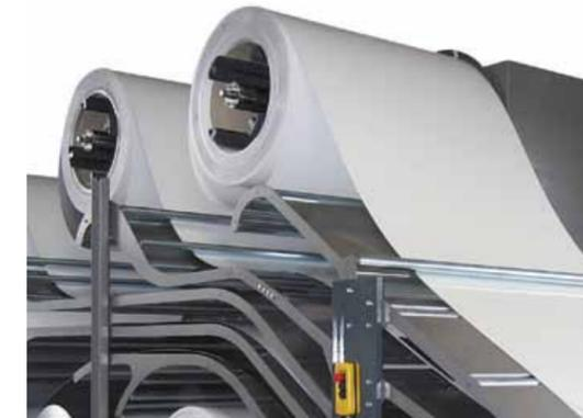
One to eight unpowered or powered decoilers from 300 up to 12000kg (26000lbs)
