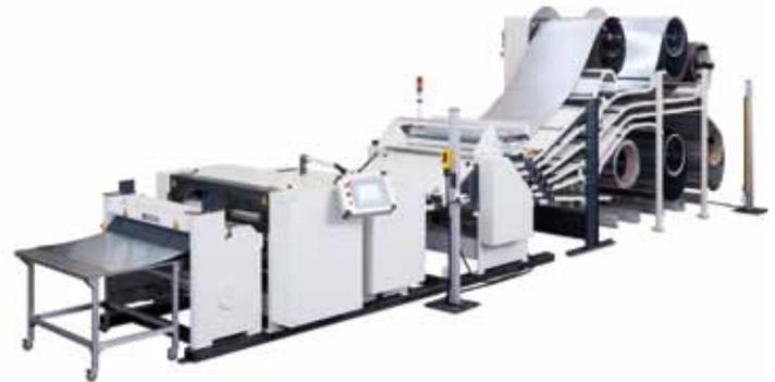
Slitting and cut to length lines - metal roofs and facades
