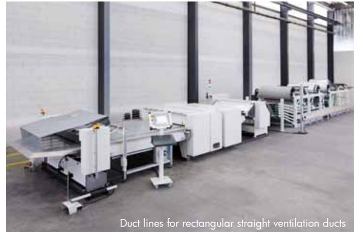
Duct lines for rectangular straight ventilation ducts
