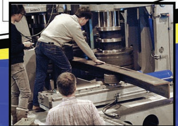
L200x200x20 in the Vertical Section Bending machine VSB3-400-3200
