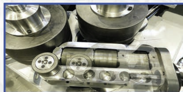
On models SB3S-XXX it is possible to have the guide rolls adjustable also in the plane of rolling. (traverse)
